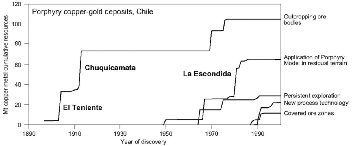
**Figure 2: Porphyry exploration in Chile: An example of the role of technical innovation in expanding the exploration search space and leading to new waves of discovery. From Hronsky and Groves (2008), based on original WMC data compiled by John Black.**
